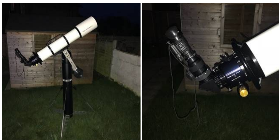
Here are a couple of photos of my 160mm refractor on the Panther TTS with the NV in afocal setup with the various adapters.
