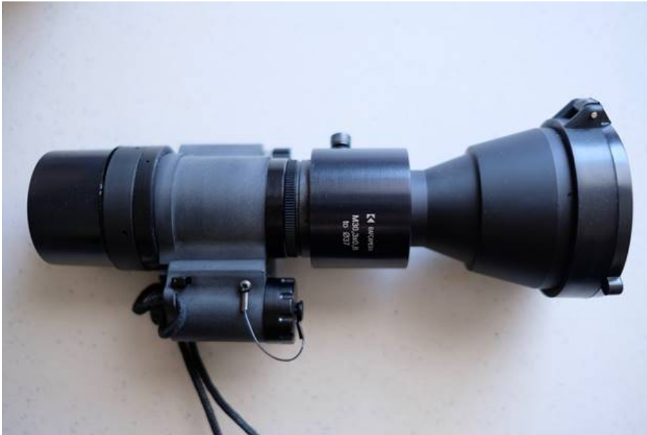
Mod3 monocular with 3x afocal lens attached
